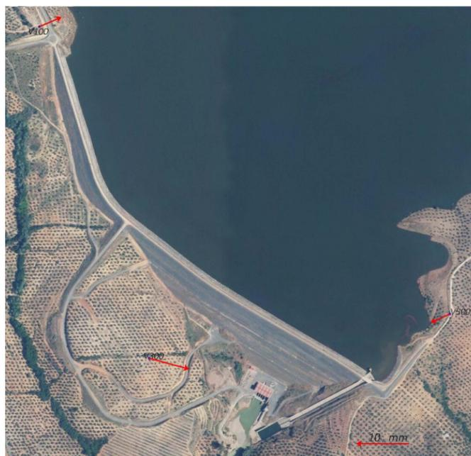
**Figure 4.** Horizontal displacements estimated at the external pillars V100, V300 and V500.
