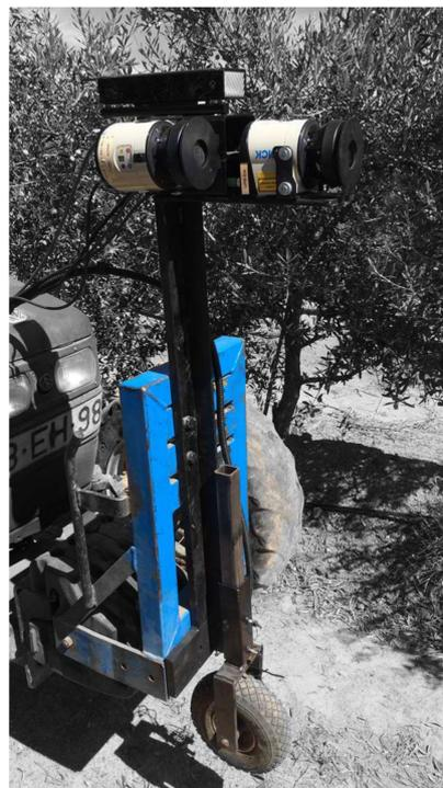
**Figure 2.** Two LiDAR sensors were mounted on the front of the tractor in different orientations to scan the olive tree structure.
