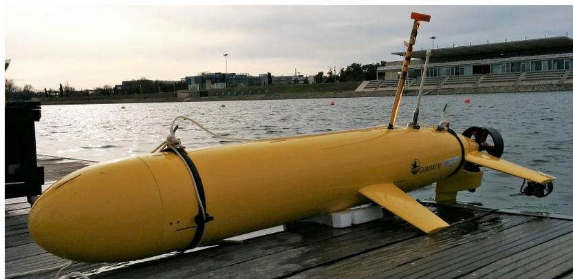
**Figure 2.** The Guanay II AUV [31] docked at the SARTI (Universitat Politècnica de Catalunya (UPC)) harbor facilities. Image taken during field tests at the Olympic Canal in Castelldefels.
