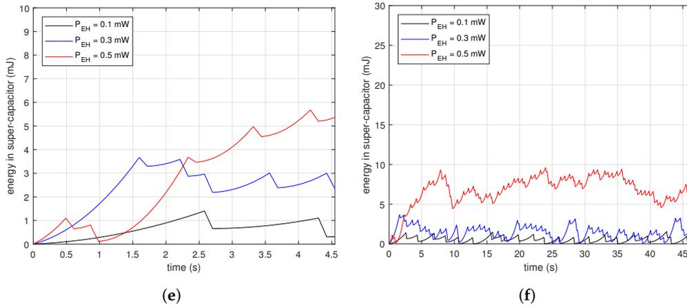
**Figure 7.** Initial amount of stored energy in a super-capacitor in conditions of  $N_{BI} = 1$ ,  $N_{BI} = 4$ , and  $N_{BI} = 8$ : (a) From 0 to 4.5 s for  $N_{BI} = 1$ ; (b) From 0 to 47 s for  $N_{BI} = 1$ ; (c) From 0 to 4.5 s for  $N_{BI} = 4$ ; (d) From 0 to 47 s for  $N_{BI} = 4$ ; (e) From 0 to 4.5 s for  $N_{BI} = 8$ ; (f) From 0 to 47 s for  $N_{BI} = 8$ .
