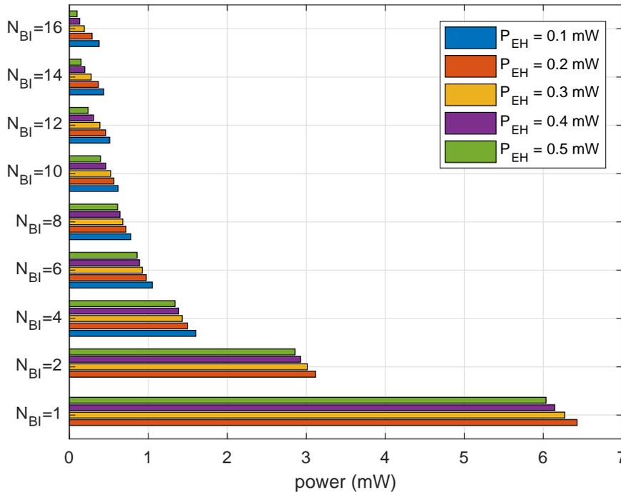
**Figure 8.** Average power consumption to recognize one beacon.
