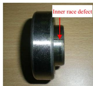
Figure 12. Bearing with inner race fault.
