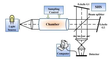
Figure 2. Structure of the visual e-nose system.
