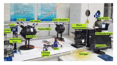
Figure 4. Experiment platform of light absorption gas detection system.
