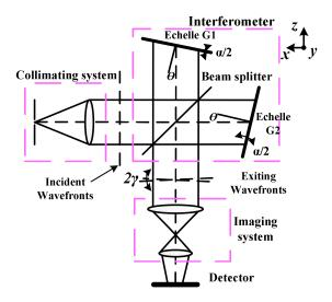
Figure 1. Structure diagram of 2D spatial heterodyne spectrometer (SHS).
