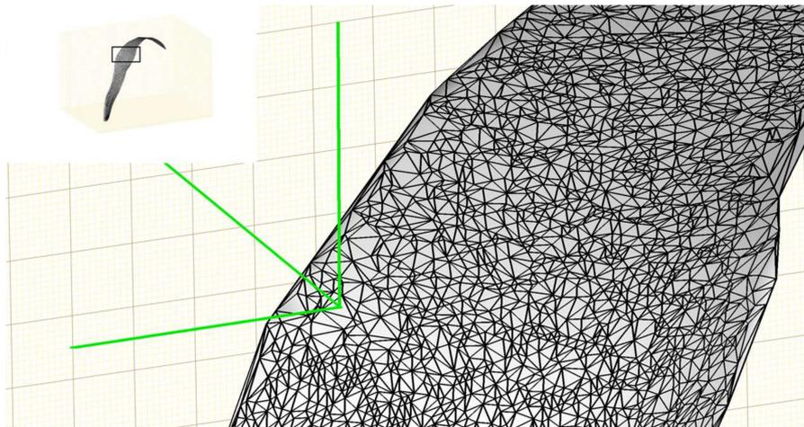
**Figure 4.** Example of triangulation of a fitted leaf surface in order to calculate leaf area, leaf inclination angle, and leaf angular distribution.
