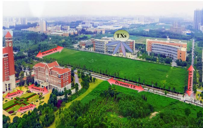
**Figure 4.** Overview of the measurement area at the campus of Shanghai Jiao Tong University, China. A spaced rectangular antenna array with 16 cross polarized patch antenna elements at the TX was placed on the rooftop of the Biomedical building during their respective measurement campaigns and a spaced uniform linear array as a user was moved around the international buildings acting as multiple-antenna user.
