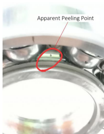
Figure 13. Peeling failure in inner ring of bearing after running for about 128 h.
