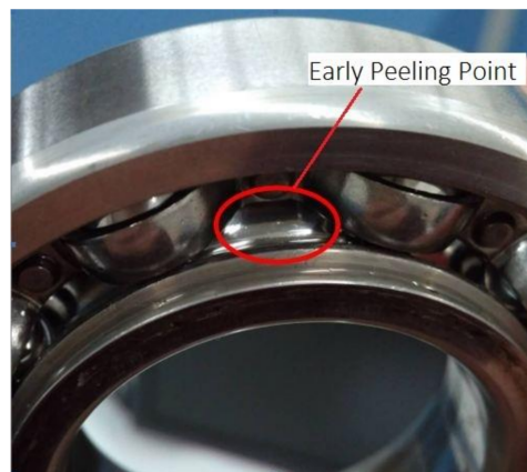
Figure 12. Early fatigue pitting failure in inner ring of bearing after running for 110 h.
