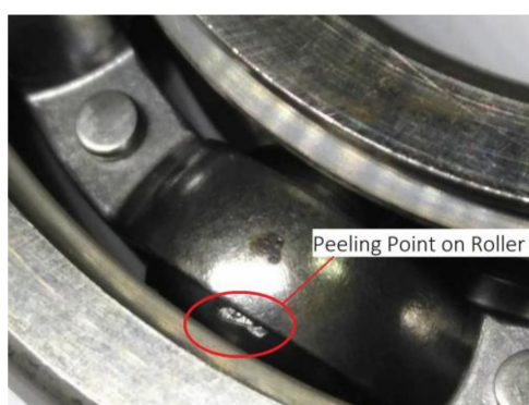
Figure 14. Peeling failure in one bearing ball after running for about 128 h.
