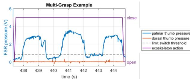
**Figure 3.** Example of a “multi-grasp” where the palmar thumb pressure crosses the limit switch threshold from below multiple times within a single exoskeleton close action, with below-threshold periods longer than 0.1 s interspersed.
