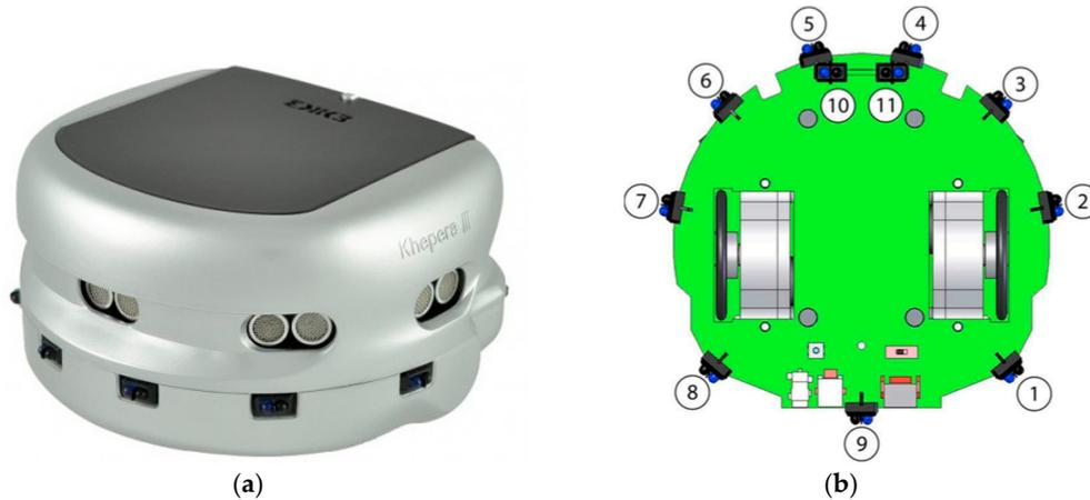
**Figure 1.** The mobile robot platform [23]: (a) Khepera III robot; (b) a bottom view of the robot showing the locations of the infrared sensor.
