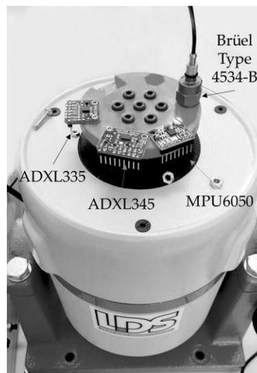
**Figure 6.** Accelerometers fixed to the electromagnetic exciter.
