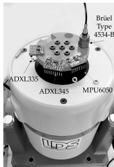
Figure 6. Accelerometers fixed to the electromagnetic exciter.
