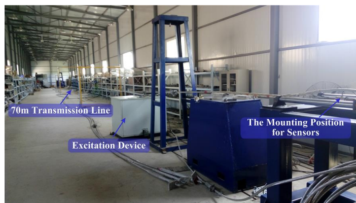
Figure 9. The setup of galloping experiment on transmission line model.
