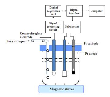
Figure 1. Acid-base coulometric autotitrator of constant current.
