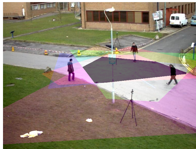
Figure 3. Visual example of the correlation between two cameras: (a) Camera 1 (camera under analysis) and detections in red color and (b) Camera 2 and detections in blue color. (c) Camera under analysis (Camera 1) with original red detections D_1 and transferred blue ones D_2 . In this case, the optimal thresholds according to the correlation between both cameras are 0.4 > \tau_1^{1,2} \leq 0.8 and 0.2 > \tau_2^{1,2} \leq 0.3 , respectively. All the images are cropped versions for visualization purposes.
