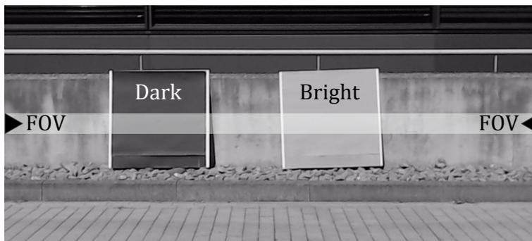
**Figure 11.** Outdoor target scene measured at 100 klx ambient sunlight including a dark and bright Lambertian target. The distance is measured along the horizontal line in the figure.
