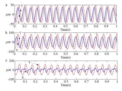
**Figure 23.** The vibration displacement signals under different running conditions. (**a**) Normal; (**b**) Rubbing; (**c**) Misalignment.
