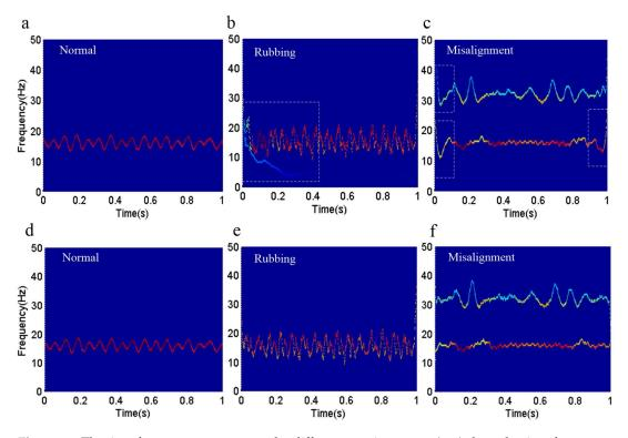
**Figure 27.** The time-frequency spectrum under different running states. (**a**–**c**) show the time-frequency spectrum of the normal, rubbing, and misalignment running states obtained by the original HHT; (**d**–**f**) show the time-frequency spectrum of the normal, rubbing, and misalignment running states obtained by the revised HHT.
