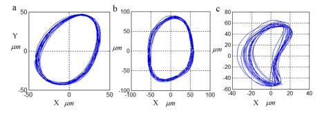
Figure 24. The axis orbits under different running conditions. (a) Normal; (b) Rubbing; (c) Misalignment.
