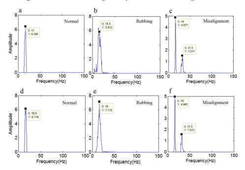
Figure 26. The marginal spectrum under different running states. (a-c) show the marginal spectrum of the normal, rubbing, and misalignment running states obtained by the original HHT; (d-f) show the marginal spectrum of the normal, rubbing, and misalignment running states obtained by the revised HHT.
