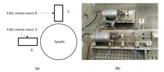
**Figure 22.** The experimental facilities. (a) The arrangement of the eddy current sensors; (b) The experimental setup.
