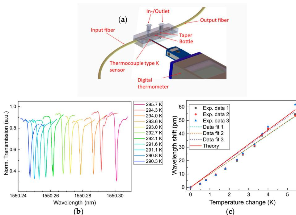
**Figure 9.** (a) Schematic of the packaged bottle resonator that includes an external digital thermometer; (b) spectral shift of a WGM resonance when temperature varies from 290.3 to 295.7 K; (c) wavelength shifts of three WGMs as a function of the temperature. Sensitivities are given in Table 3.
