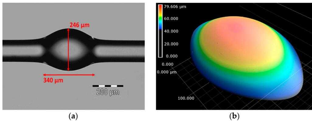
**Figure 1.** (a) Microscope image of the glass bottle resonator (central diameter ( $D_c$ ) = 246  $\mu\text{m}$  and length ( $L$ ) = 340  $\mu\text{m}$ ) fabricated with a soften and compress technique; (b) the corresponding laser-scanned microscope image of the bottle surface.
