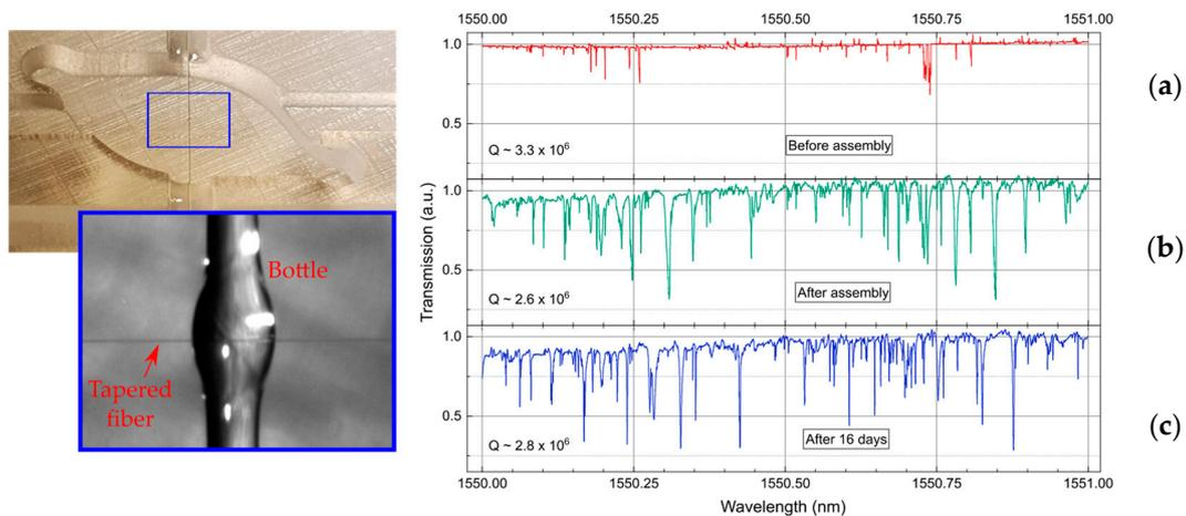
**Figure 8.** Optical characterization of the packaged bottle: (a) before assembly; (b) after assembly; and (c) after 16 days.
