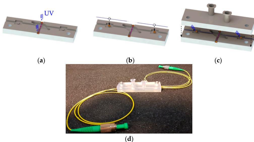
**Figure 7.** (a–c) Assembly process of a bottle resonator; (d) first 3D-printed package of a taper-bottle system.
