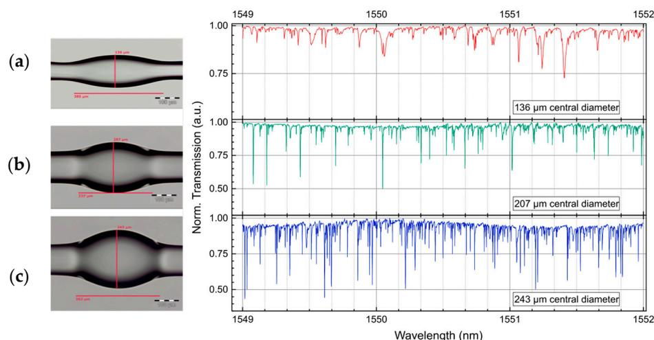
**Figure 6.** Transmission spectra obtained with three different bottle structures when a  $5 \mu\text{m}$  diameter is located in the center. Bottle parameters are (a)  $D_c = 136 \mu\text{m}$ ,  $L = 385 \mu\text{m}$ ; (b)  $D_c = 207 \mu\text{m}$ ,  $L = 337 \mu\text{m}$ , and (c)  $D_c = 243 \mu\text{m}$ ,  $L = 363 \mu\text{m}$ . Step size was  $0.1 \text{ pm}$ .
