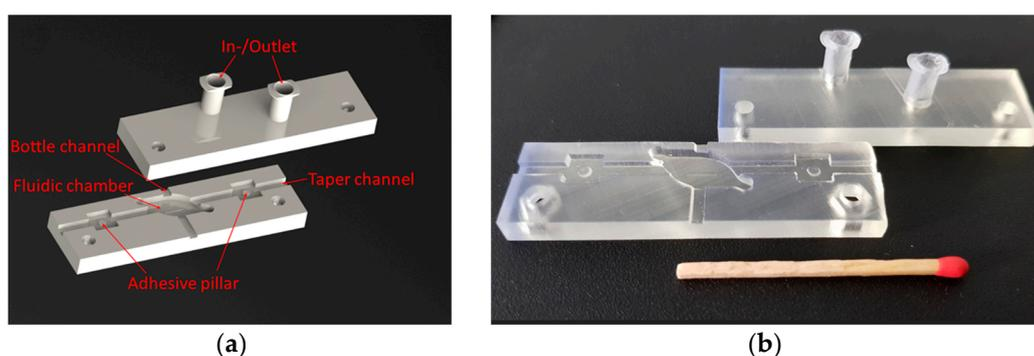
**Figure 3.** Package for bottle resonators: (a) CAD design and (b) 3D printed plastic package.
