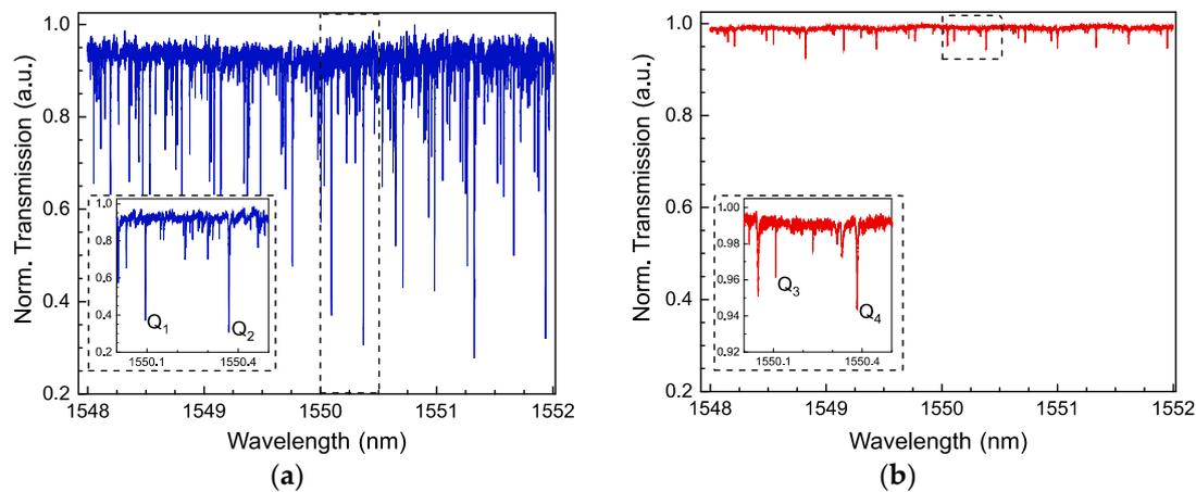
**Figure 5.** Transmission spectra of a bottle ( $D_c = 243 \mu\text{m}$  and  $L = 363 \mu\text{m}$ ) interrogated with two taper diameters of (a)  $5 \mu\text{m}$  and (b)  $6.6 \mu\text{m}$ . Zoomed plots show some WGMs where quality (Q) factors were found to be  $Q_1 \sim 1.91 \times 10^6$ ,  $Q_2 \sim 7.7 \times 10^5$ ,  $Q_3 \sim 7.38 \times 10^6$ , and  $Q_4 \sim 4.4 \times 10^5$ . Step size was  $0.1 \text{ pm}$ .
