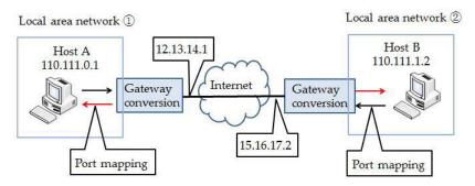
Figure 4. The schematic of intranet penetration technology.
