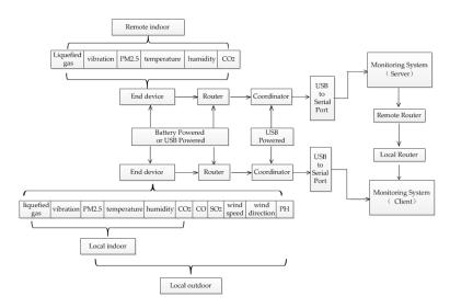
Figure 1. The layout of overall system.
