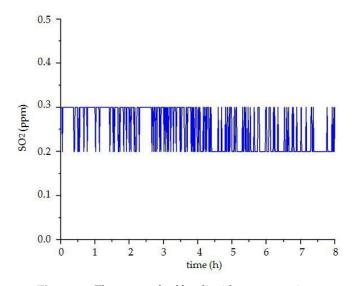
Figure 25. The curve of sulfur dioxide concentration.
