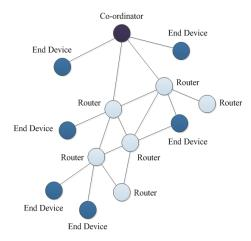
Figure 3. The schematic of mesh topology.
