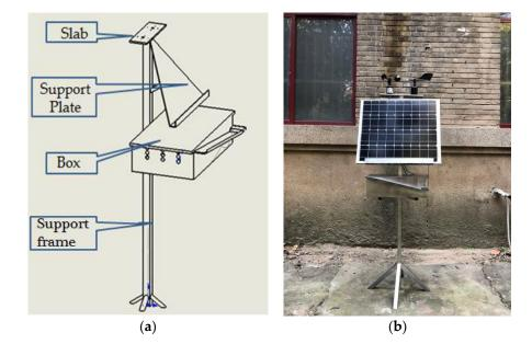
**Figure 7.** The design of outdoor package device: (**a**) picture of the structure; (**b**) picture of the real product.
