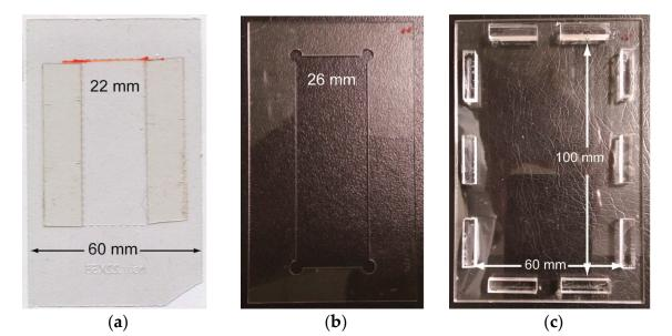
Figure S4. The parts of an alignment template. (a) Film support; (b) Slide frame; and (c) Holder.
