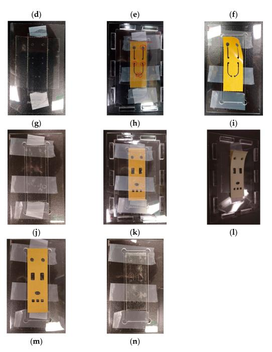
**Figure S5.** Pictures showing the steps of aligning and stacking units of double adhesive and transparency films to form a microfluidic chip.
