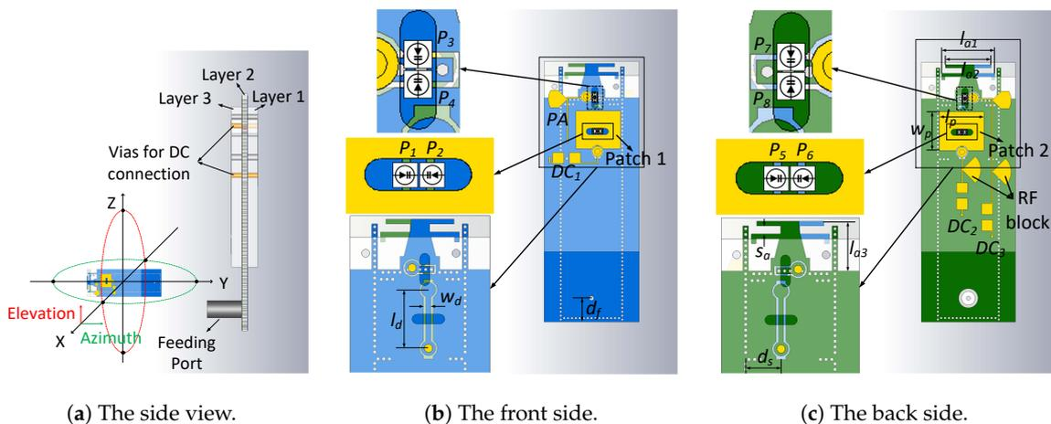
**Figure 2.** The structure of proposed antenna.
