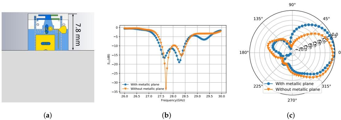
**Figure 9.** The influence of adjacent metallic plane: (a) the array element with a metallic plane above; (b) the  $S_{11}$  of Broadside 1 with or without the metallic plane; and (c) the radiation pattern of Broadside 1 with or without the metallic plane.
