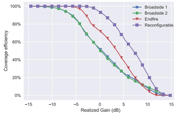
Figure 13. Coverage efficiency of the RPA and every single mode.
