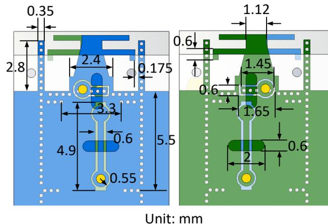
Figure A1. The detailed dimensions of the proposed RPRA.
