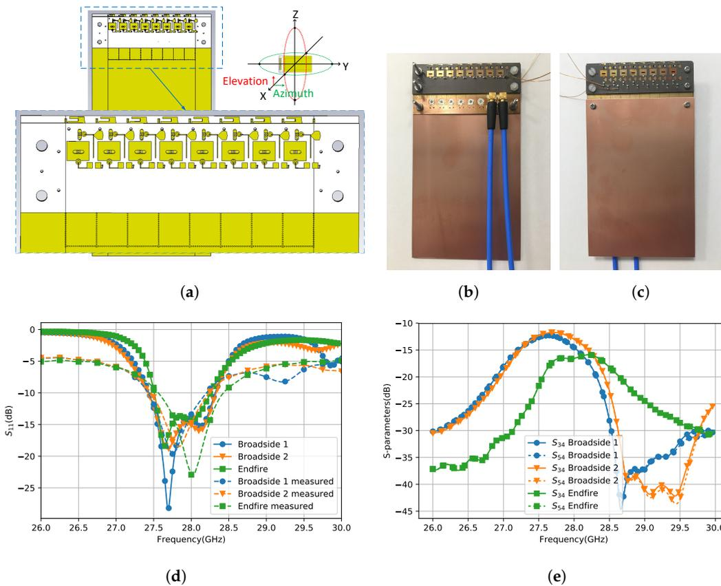
**Figure 8.** The array structure and the experiment results of the middle element: (a) the array structure of the front view; (b) front view; (c) back view; (d) the simulated and measured reflection coefficient of the middle element; and (e) the simulated mutual coupling of the middle element.
