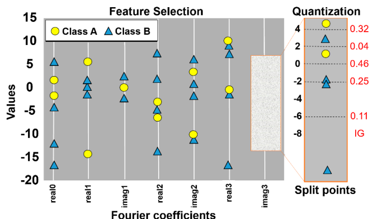
Figure 14. Example of how the SFA-W discretization process works. In this example, two classes are used ‘A’ and ‘B’, with the real0 and imag3 coefficients selected as the best. Then, the best cut-off point was 0.46.
