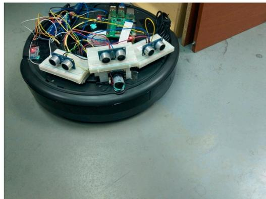
**Figure 17.** Three ultrasonic sensors installed on the clean robot.
