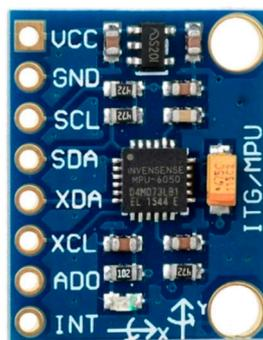
Figure 8. MPU-6050 six-axis sensor.
