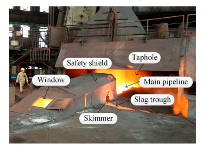
Figure 2. Real casthouse of No. 2 BF in an ironmaking plant.
