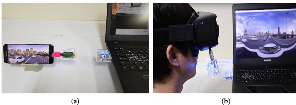
**Figure 20.** Implemented mobile VR 360-degree video player using mmWave communication; (a)  $3840 \times 1920$  full picture consisting of 9 tiles; (b) one extracted tile of 9 tiles.
