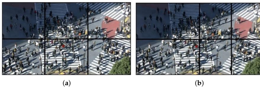
Figure 14. Tile partition of *PeopleOnStreet* test sequence with (a) conventional uniform tile partitioning, (b) Proposed non-uniform tile partitioning method considering Samsung Galaxy S7 Edge environments.
