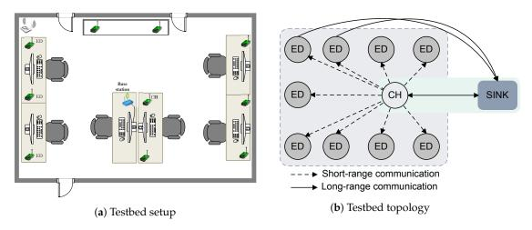
Figure 7. Network topology and indoor testbed deployment.
