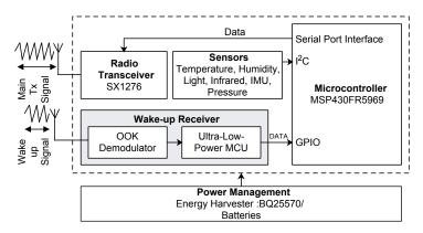
Figure 6. Hardware architecture of the heterogeneous communication mote used for testbed evaluation.
