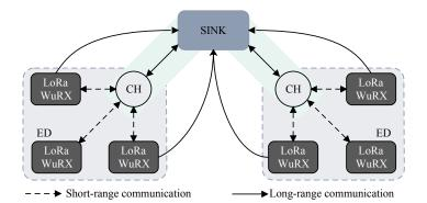
Figure 3. Heterogeneous IoT topology for sensor and actuator networks.
