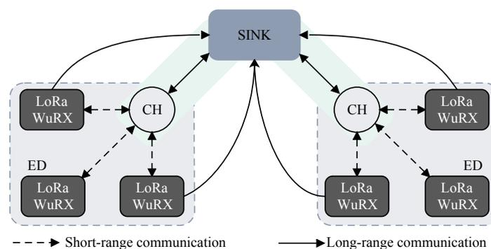
**Figure 3.** Heterogeneous IoT topology for sensor and actuator networks.
