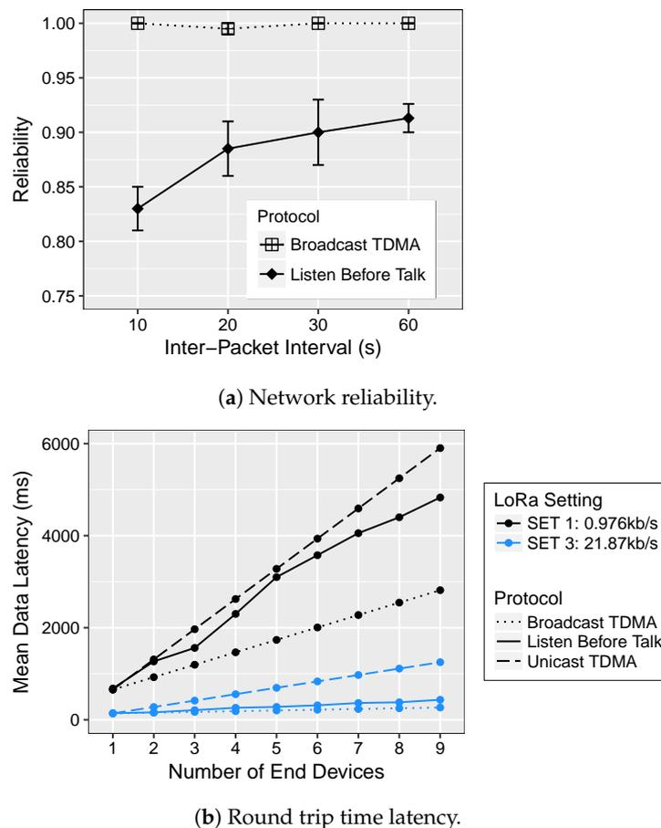
**Figure 9.** Network reliability and latency evaluation using different LoRa radio setting and protocols.
