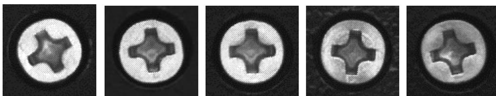
**Figure 4.** Defect-free screws.
