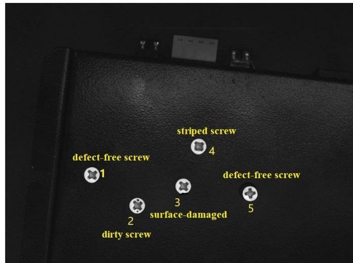
Figure 14. Screws for testing.
