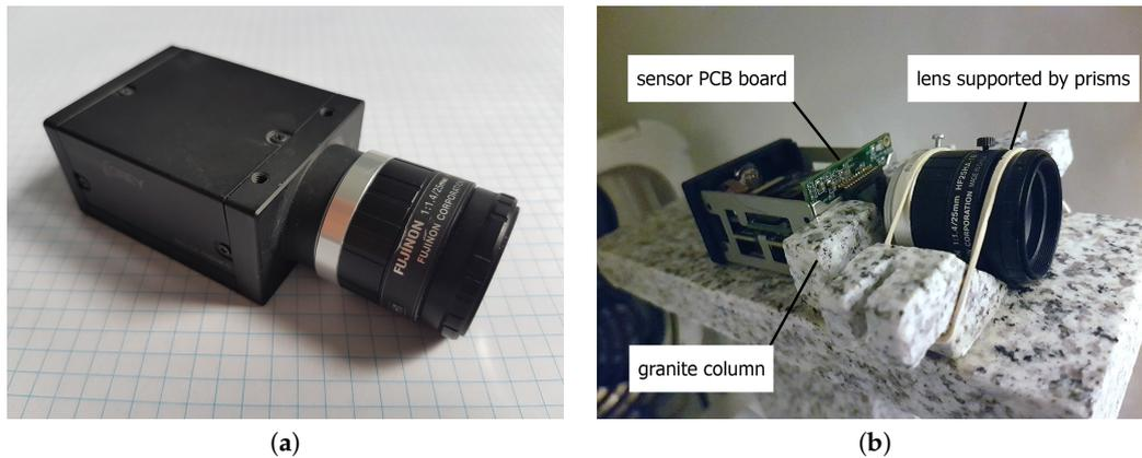
**Figure 7.** The original and modified camera unit. (a) The original camera unit. (b) A photo of the modified camera. The lens is positioned on two granite prisms while the sensor is supported between two granite columns and can only translate along the vertical sensor axis and rotate around the horizontal sensor axis.
