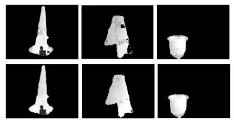
**Figure 9.** Optimization results of the disparity maps, where the basic disparity maps and the optimization results of the least squares plane fitting interpolation method are given in the first row and second row, respectively.
