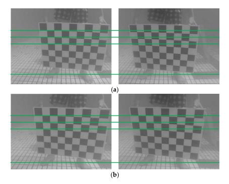
**Figure 4.** Comparison of the left and right images before and after correction. (**a**) The left and right images before correction; (**b**) The left and right images after correction.
