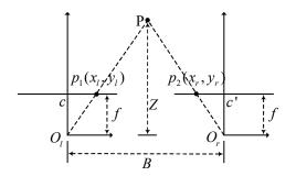
Figure 11. Diagram of binocular vision measurement principle.
