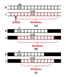
**Figure 8.** Comparison of disparity calculation. (**a**) The stereo matching principle of SGM algorithm; (**b**) Stereo matching without constraint of the valid target area; (**c**) Stereo matching strictly constrained within the valid target area.
