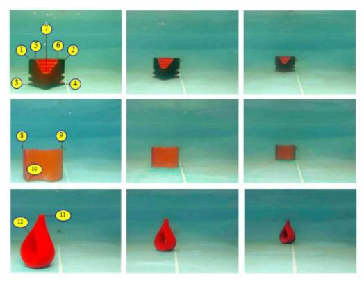
**Figure 14.** Underwater targets with observed points marked for distance measurement, the distances are about 1 m, 1.5 m and 2 m from left to right.
