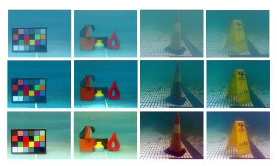
**Figure 5.** Comparison of the original underwater images, the results using the method in Reference [38] and the results using BM3D filtering and color correction, where the first row shows the original underwater images, the second row shows the results using the method in Reference [38] and the third row shows the results using BM3D filtering and color correction.
