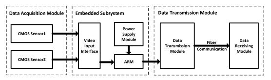
Figure 2. System hardware diagram.
