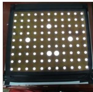
**Figure 6.** Target for binocular vision calibration.
