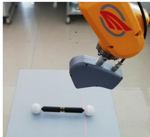
**Figure 15.** The measurement of ball arm by AAMS.
