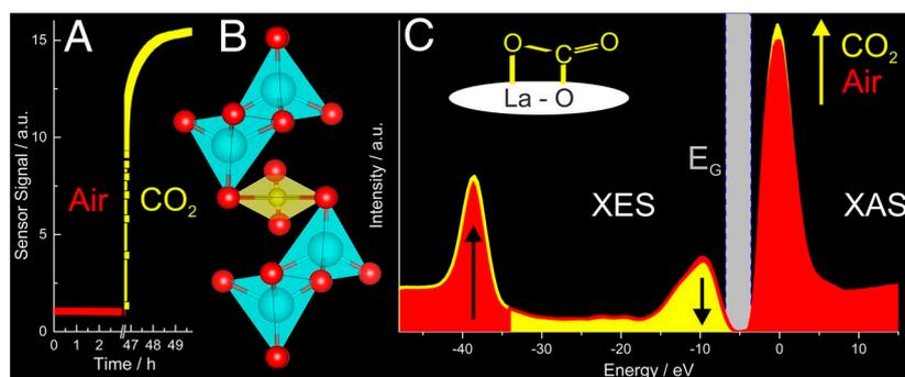
**Figure 3.** Operando spectroscopic study of  $La_2O_2CO_3$  during  $CO_2$  (10,000 ppm) sensing in 50 %r.h. at  $250$  °C: (A) Sensor signals, (B) schematics of the unit cell of  $La_2O_2CO_3$  (La = cyan, O = red, C = yellow) and (C) XES and XAS spectra before (red) and during (yellow)  $CO_2$  exposure. Figure is reprinted from reference [38].
