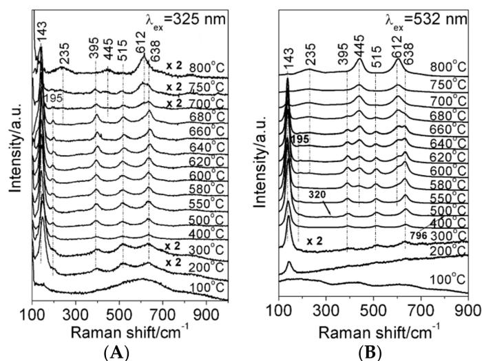
**Figure 4.** Raman spectra of TiO<sub>2</sub> calcined at different temperatures. (A) The spectra were recorded with an excitation at 325 nm, (B) with 532 nm. Reprinted with permission from The Journal of Physical Chemistry B, reference [63]. Copyright 2006 American Chemical Society.
