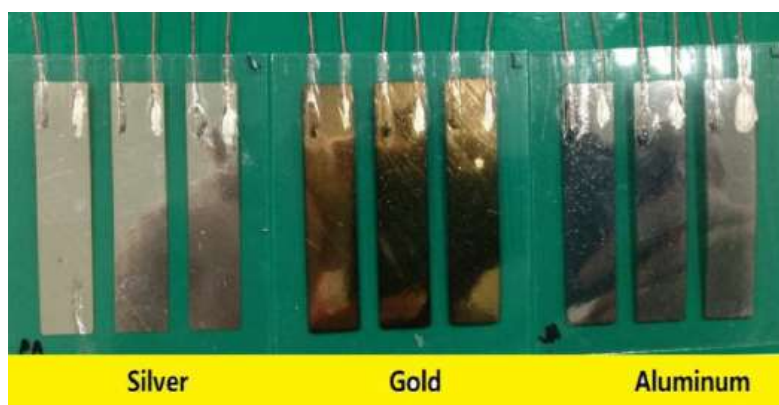
Figure 16. Fabricated gold, silver and aluminum electrode electroactive paper specimens [81].
