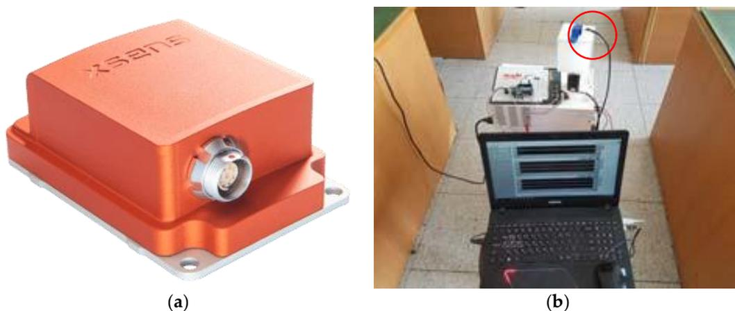
**Figure 6.** Wi-Fi and geomagnetic signal collection positions and structure for creating the radio map: (a) Geomagnetic sensor for experiment; (b) experimental system for collecting the geomagnetic and Wi-Fi signals.
