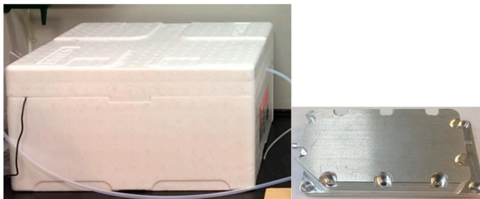
**Figure 2.** Sample chamber (left) and sensing chamber (right).
