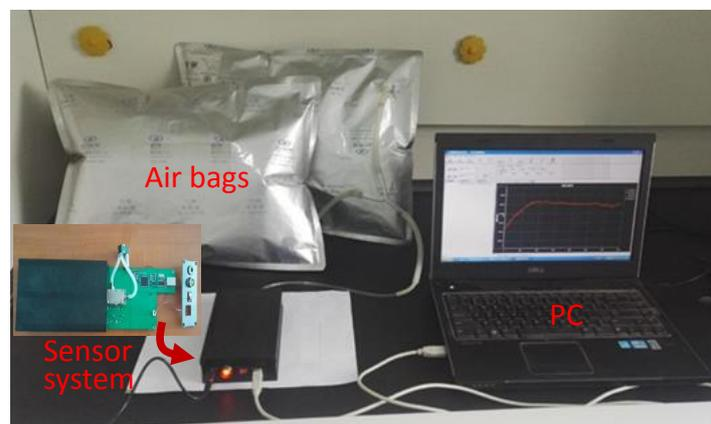
Figure 11. The experimental setup for characterizing the proposed Love wave sensor.
