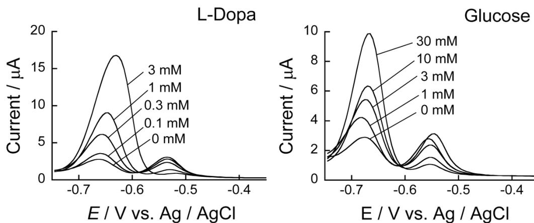
DPVs of the ARS-confined (PBA-PEI/CMC)<sub>10</sub>PBA-PEI film-coated electrodes in the absence and presence of L-dopa (0.1-3 mM) and glucose (1-30 mM) at pH 9.0.
