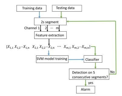
**Figure 2.** Block diagram of seizure detector training and testing (*m*: number of channels; *n*: number of features of each channel).
