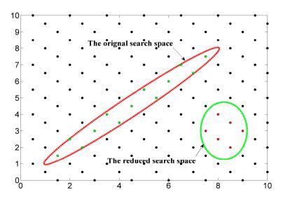
Figure 2. The effect of lattice reduction on the searching space.
