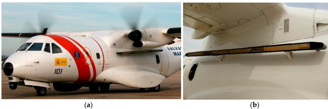
**Figure 1.** (a) Aircraft belonging to Spanish government used to acquire SAR images; (b) Detail of SLAR Terma-sensor antenna, which are 12 ft in dimension.
