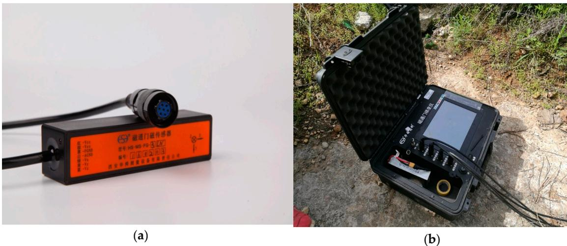
**Figure 15.** (a) Three-component fluxgate sensor of HS-MS-FG-3-LN; (b) Data acquisition card of NI 9239.
