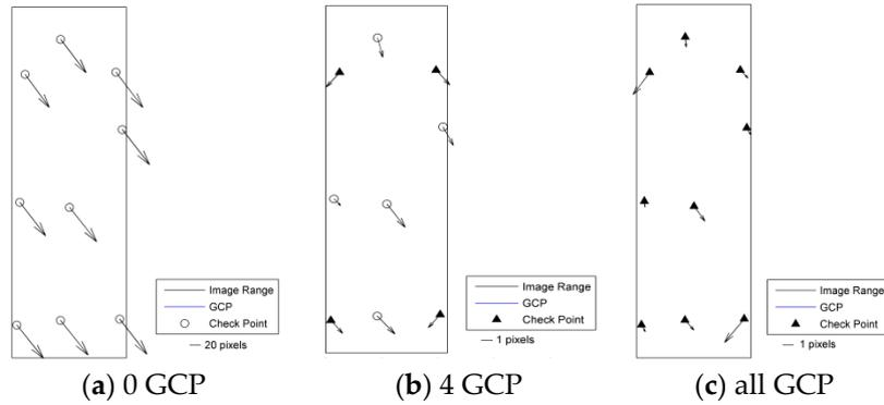
**Figure 3.** Residual distributions of check points of the SL mode orientation for Taiyuan. (a) 0 GCP; (b) 4 GCP; (c) all GCP.
