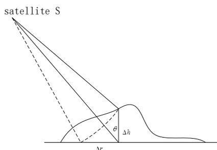
**Figure 1.** Positioning error caused by topographic relief.
