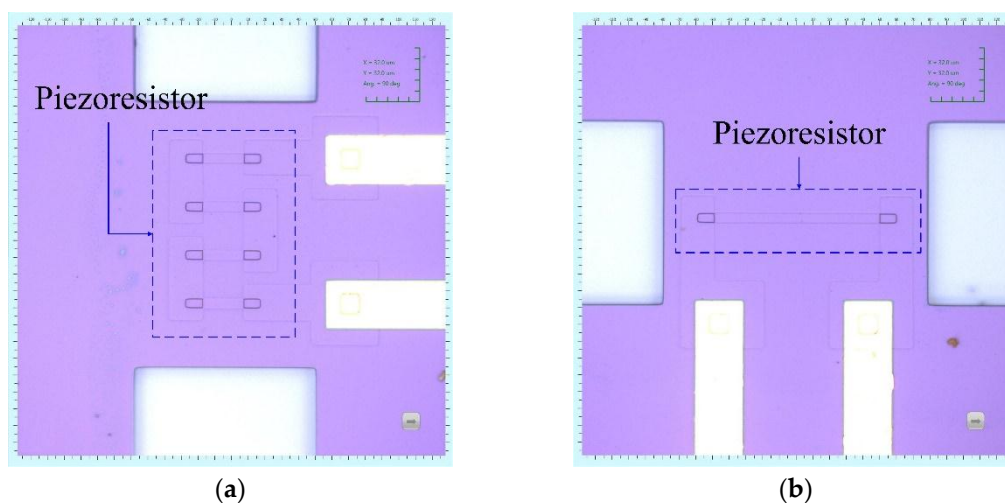
Figure A2. Microscopic photos of piezoresistors in two patterns: (a) piezoresistor in position 1 shown in Figure 16; (b) piezoresistor in position 2 shown in Figure 16.
