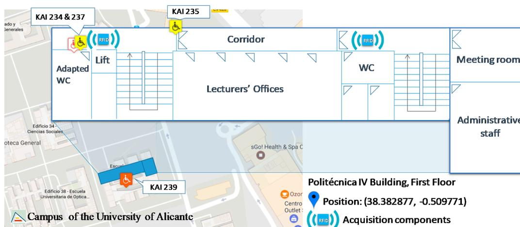
Figure 14. Indoor scenario and RFID-based acquisition components deployed.
