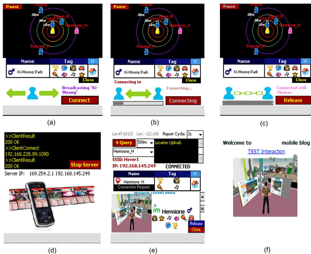
**Figure 4.** Screenshots of *T-Wing* on an embedded platform: (a) Searching nearby users; (b) Connecting over Wi-Fi network interface; (c) Established connection over Wi-Fi in a peer-to-peer manner; (d) *T-Wing* web provider with log messages; (e) Miniaturized web page; (f) Web browsing with rich content.
