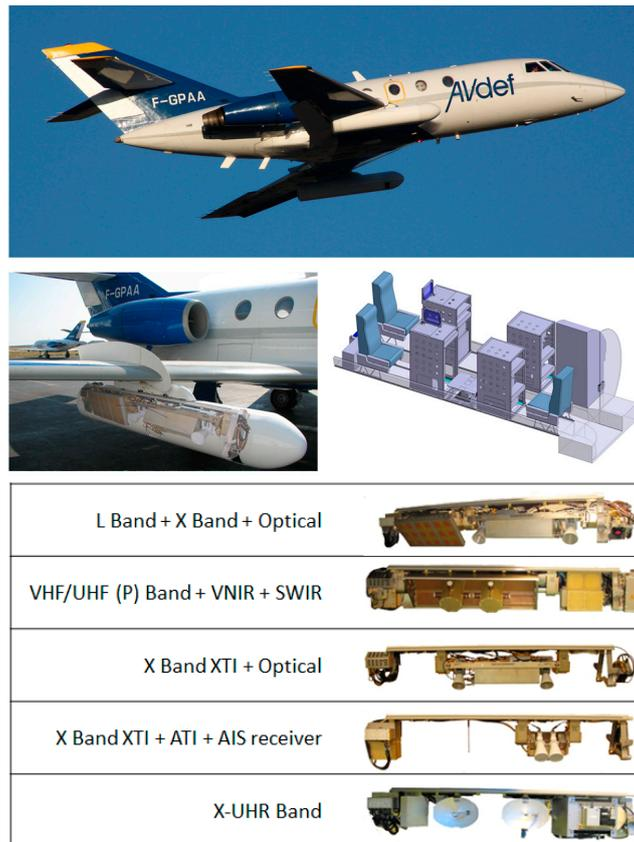
Figure 2. SETHI platform (aircraft, pod and cabin layout) and in-pod payload configuration examples.
