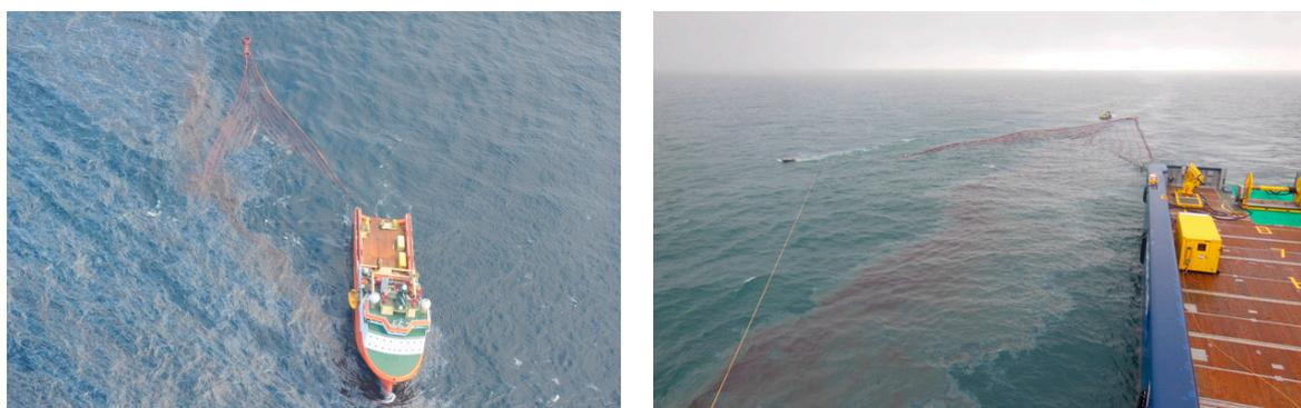
**Figure 1.** MOS Sweeper [10] mechanical recovering system operated by NOFO during trial at sea (photographs provided by NOFO).
