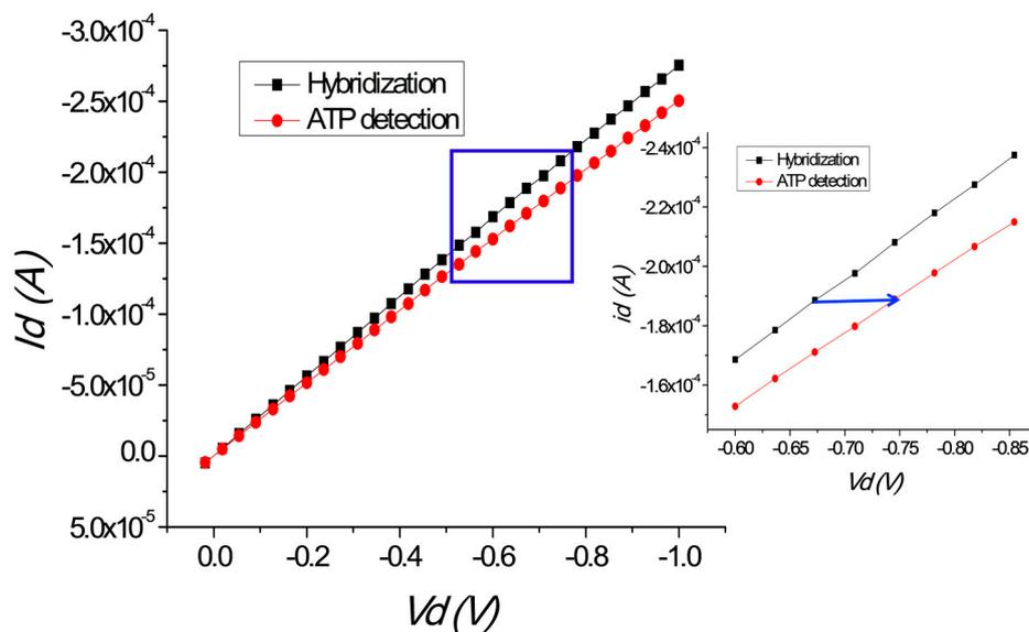
**Figure 7.**  $I$ - $V$  (drain current  $I_d$  and drain-source voltage  $V_d$ ) characteristics of the modified diamond-based field-effect transistor (FET) showing ATP activity (gate voltage  $-0.2$  V).
