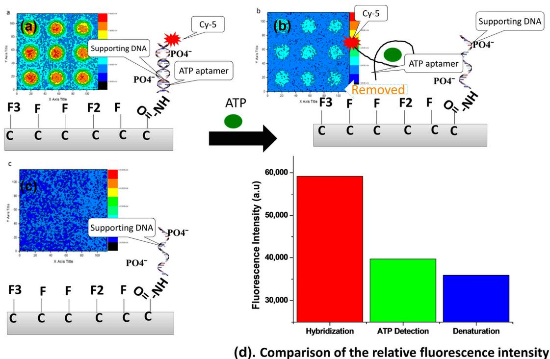
**Figure 5.** Fluorescence signals at different steps of the sensor operation. (a) Hybridization of the supporting DNA with the aptamer modified with Cy-5 as a fluorescent indicator; (b) ATP detection via the aptamer; (c) Denaturation, which occurred when ATP and the aptamer were removed from the sensor and the DNA became single stranded; (d) Comparison of the relative fluorescence intensities at the three observation points for similar areas.
