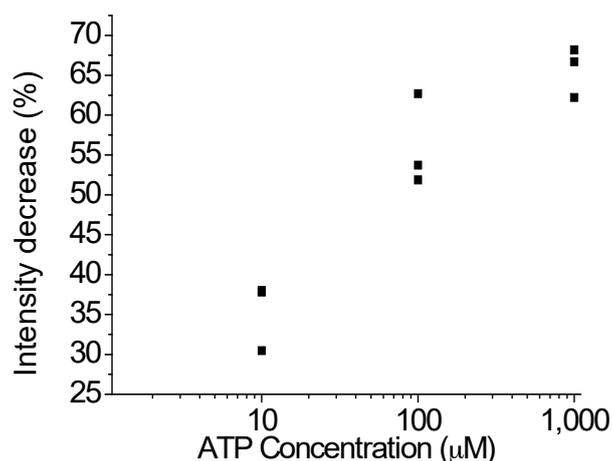
**Figure 6.** Relationship between the fluorescence intensity for different ATP concentrations. Every single data point is the average of three measurements.
