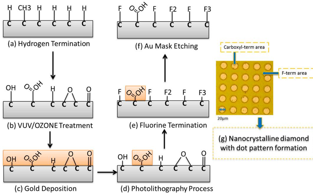
**Figure 1.** Schematic diagram of micropattern fabrication on the nanocrystalline diamond (NCD) surface. (a) Hydrogen termination; (b) Vacuum ultraviolet (VUV)/Ozone treatment; (c) Gold deposition; (d) Photolithography process; (e) Fluorine termination; (f) Au mask etching; (g) Optical microscopy image of the dot pattern formed on the NCD surface. The dots are terminated by carboxyl groups and regions outside the dots are fluorine-terminated as a background.
