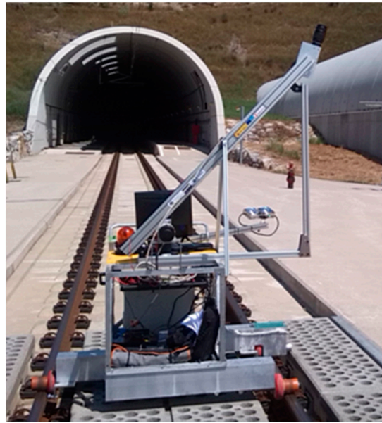
Figure 5. Prototype of the tunnel inspection platform.
