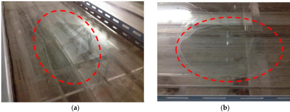
**Figure 18.** Defect in the model bridge: (a) Overall view of the bridge deck; (b) Detail view of the defect in the bridge deck.
